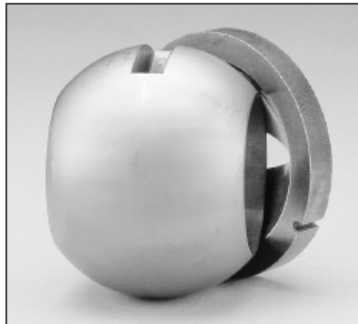
316 sintered metal seats are impregnated with TFE or graphite to provide positive shut-off and eliminate galling when contacting the hard coated ball.
